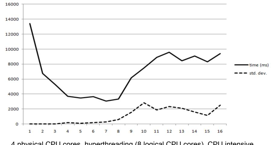
4 physical CPU cores, hyperthreading (8 logical CPU cores), CPU intensive operations with floating point arithmetics
